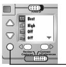
1 With the camera on, set the Slider switch to Preferences.
