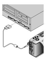
Serial ports are usually labeled COM1 and COM2, or A and B. If your computer has a 25-pin port, you need to use a 9-pin adapter (available at your local computer store) and attach it to the port before attaching the serial cable to the computer.
