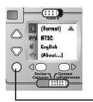
1 With the camera on, set the Slider switch to Preferences.
